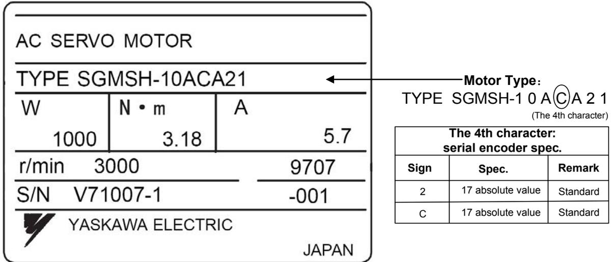
Fig. 6-2 Name plate of servo motor-encoder resolution
