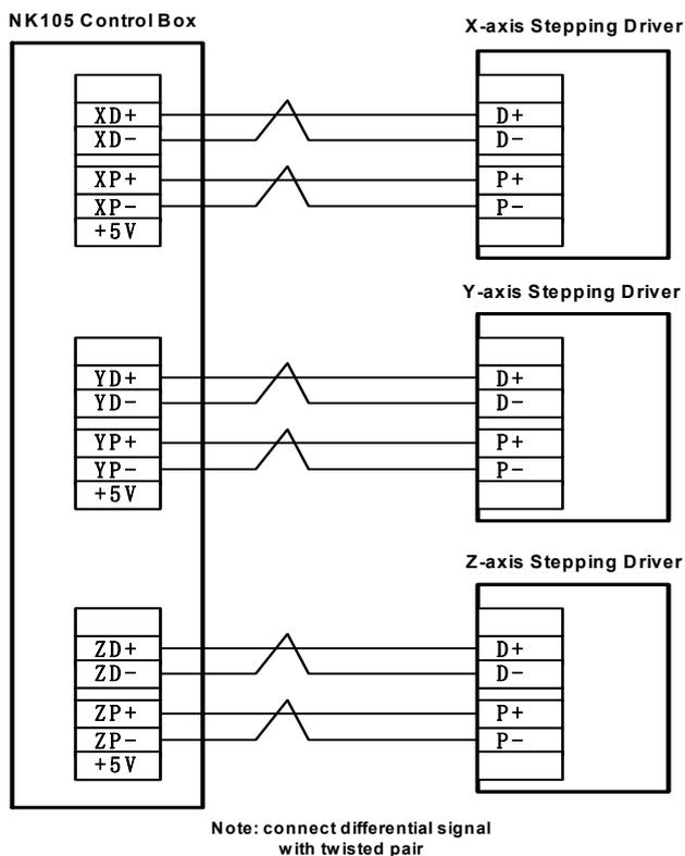
Fig. 9-1 Wiring of NK105 control box and stepping driver of differential input
