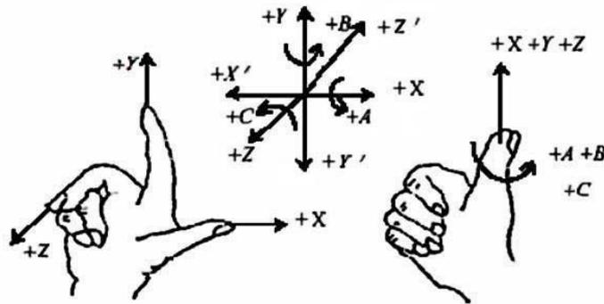
Fig. 4-1 The coordinate system conforming to right-hand rule
