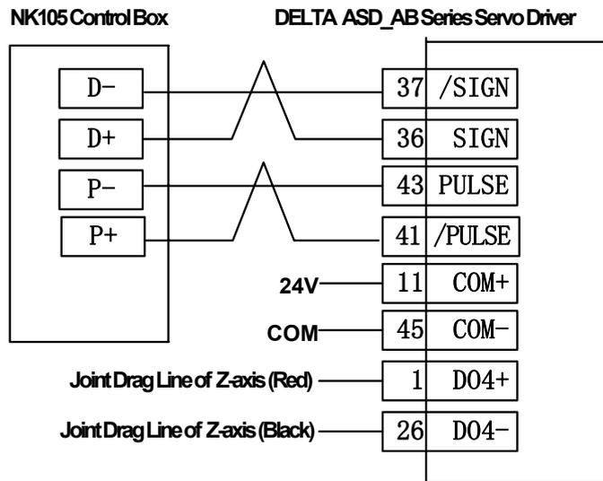
Fig. 9-4 Wring diagram of NK105 and DELTA ASD\_AB driver
