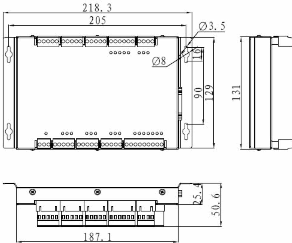
Fig. 1-1 Dimension drawing of NK105 control box
