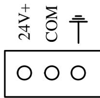
Fig. 2-2 Pin definition of +24V power input interface
